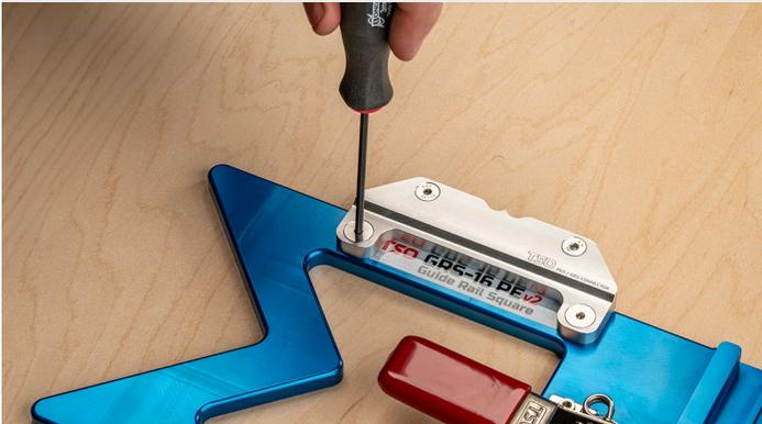
**Step 2.** Loosen the torpedo nut on the underside of the *Guide Rail Square Connector* and slide the *Parallel Guide Track* through it.
