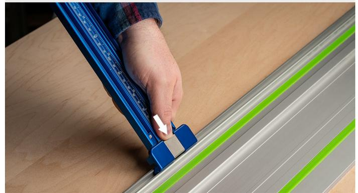
**Step 3.** Continuing to keep the button depressed, tilt the parallel guide downward until it lays flat. Once flat, release the button.
