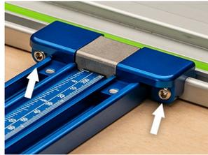
**Step 1.** With the parallel guide attached to your guide rail and laying flat, use the provided *3mm Hex Driver* to slowly tighten one of the nylon-tipped adjustment screws. While doing so, keep an eye on the far end of the *Parallel Guide Track*.
