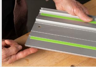
The splinterguard edge must align perfectly with your saw's kerf, as repeated use can cause wear. To check, make a test cut and feel along the splinterguard and workpiece. If the workpiece edge extends past the splinterguard, renew it.
