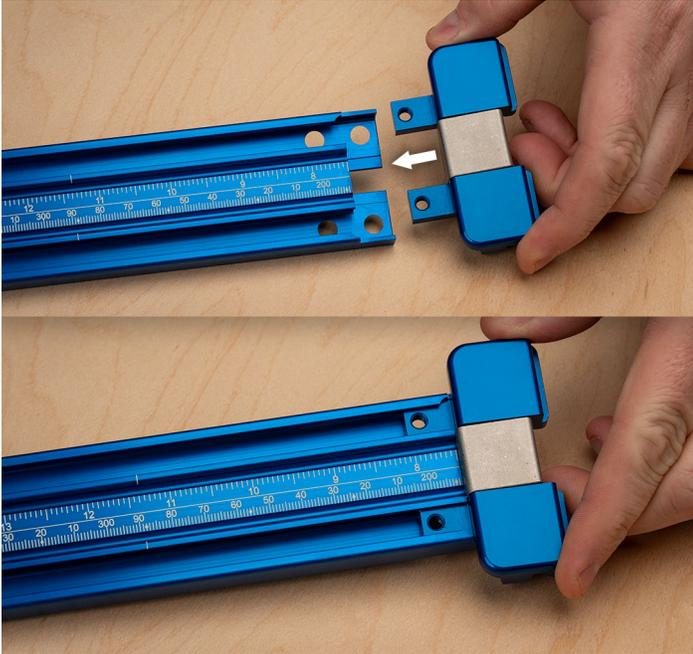
**Step 2.** Using the included *3mm Hex Driver*, attach the *Drop-Loc Connector* to *Parallel Guide Track* using four of the included *Flat Head Screws*. Ensure screw heads are flush or below the surface of the track. Hand tighten.
