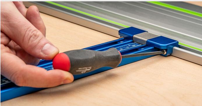
**Step 2.** As the screw is tightened, the end of the *Parallel Guide Track* will lift off your work surface slightly.
