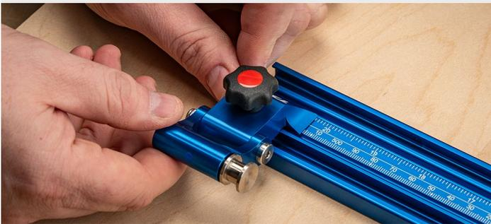
**Step 2.** Position the cursor to a desired calibration dimension (e.g. 10") and tighten the knob of the *Flip Stop Pro* to prevent movement during calibration.
