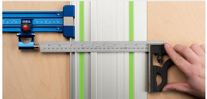
**Step 4.** Using the included 3mm Hex Driver, turn the calibration plunger on the *Flip Stop Pro* arm (clockwise to extend and counterclockwise to retract) until the plunger meets the reference surface. The *Flip Stop Pro* is now calibrated. Repeat for additional *Flip Stop Pros*.
