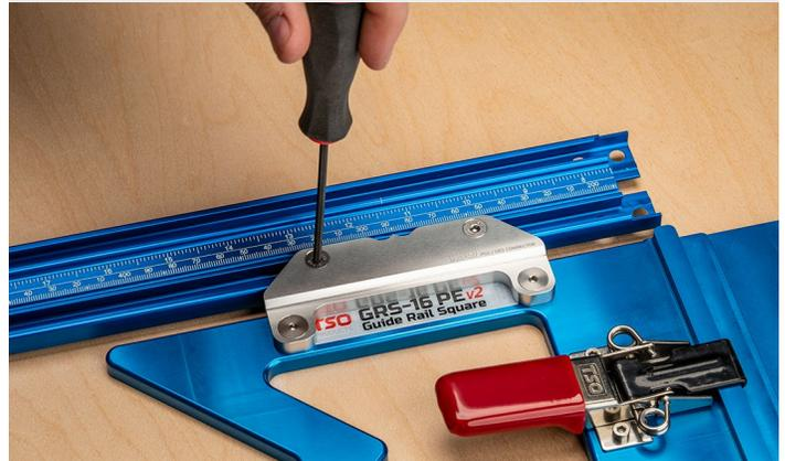
**Step 5.** Mount the *GRS-16* to your guide rail and install *Flip Stop Pro*.
