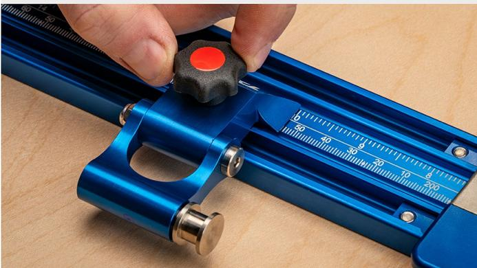
**Step 3.** Using a trusted measurement instrument (e.g. combination square or double square), set it to the same dimension you selected in Step 2. Extend the square over the guide rail and place its reference edge firmly against the splinterguard, ensuring the tool blade remains perpendicular to the guide rail. *Note: If you don't have access to a tool for calibration, a panel cut to a known accurate size (e.g. 10" x 10") is an acceptable alternative.*
