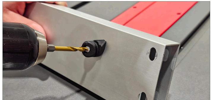
Step 1H. Drill out the Rivet holding on the Push Stick Storage Mount on back of SawStop Fence Extrusion
